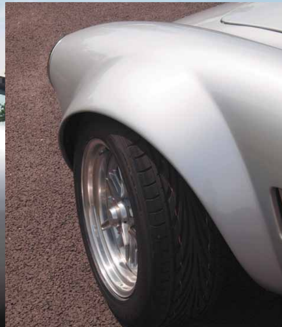
A distinctive aspect of the Cobretti body is the wide, flat top wing which resulted from increasing the car's width to suit the wider Ford Granada front subframe.
