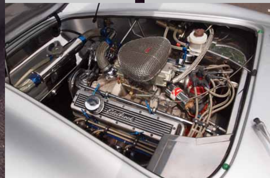
The engine bay is exactly what you would expect to see and demonstrates the same level of quality finish as the whole car. It's a Chevy 350 offering 360 bhp.
