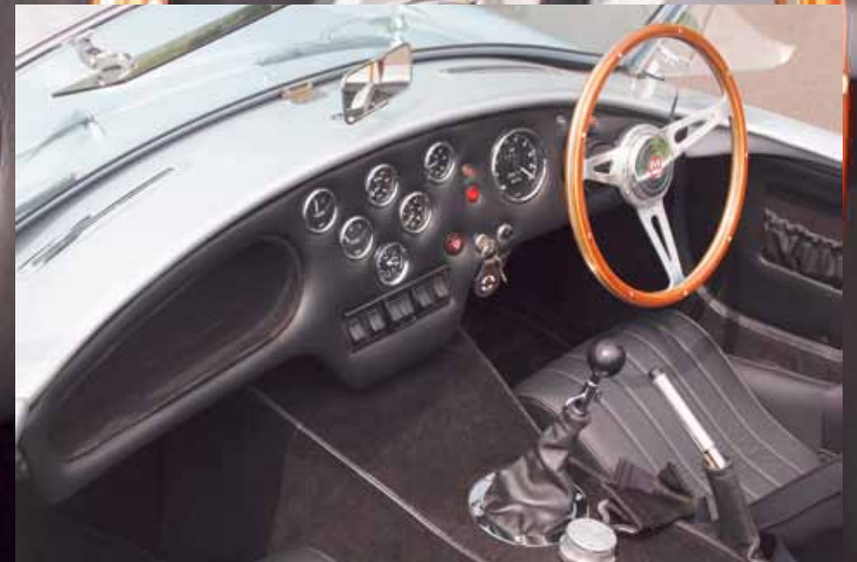
The interior is comfortable and adheres to the Cobra norm. Switches are from the Jaguar to comply with IVA but the owner may change them.
